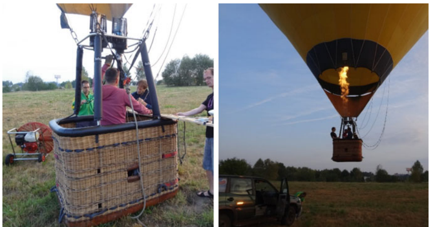
Fig. 3.75 Mounting GNSS antenna and meteorological sensors on the balloon basket (left) and the balloon during ascending (right)
