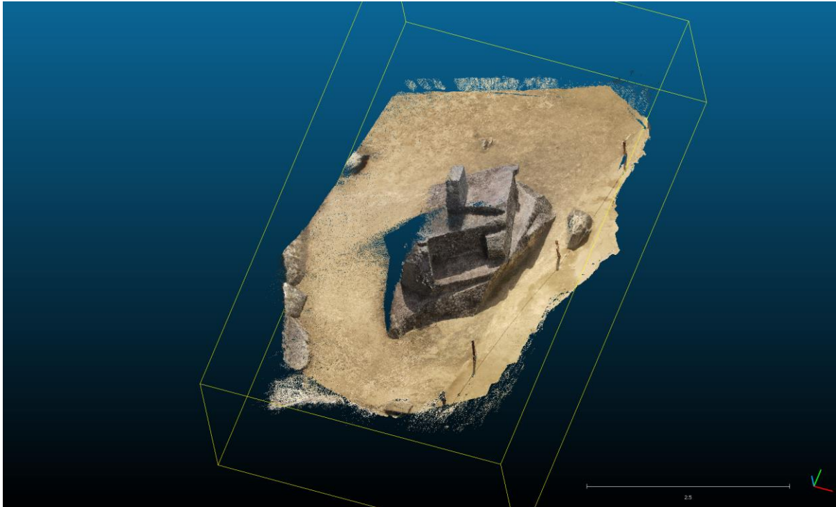
Figure 2. Three-dimensional model of Intihuatana stone, acquired and georeferenced with the same cellular phone.
