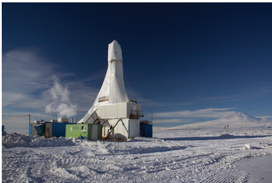
Figure 2. ANDRILL (Antarctic Geological Drilling) rig in late 2007 (Southern McMurdo Sound, SMS Project), operating on floating sea ice (~8.5 m thick) platform.
