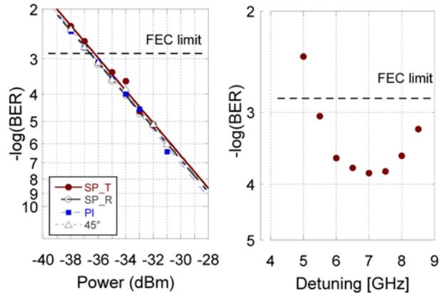
Fig. 2. Single channel B2B results. (a) BER vs. received power for horizontal fixed linear polarizations: horizontal (red dots), vertical (white dots), 45 degrees (white triangles) and in PI configuration (blue squares). (b) BER vs. detuning, for  $-34$  dBm received power.
