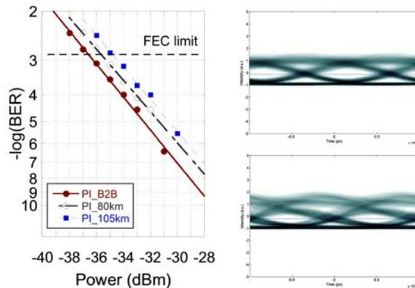
Fig. 3. Single channel results. (a): BER vs. received power in back to back (red dots), after 80 km (white dots), and 105 km (blue squares) transmission. (b): eye diagrams at  $-30$  dBm received power in back to back (upper) and 105 km transmission (lower).
