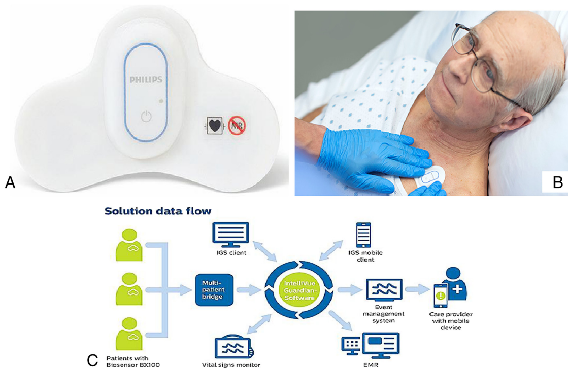
Figure 29: BX100 Philips Biosensor (Philips, 2019): front view of the device (a), and its application on a patient (b), the graphical scheme of the health monitoring system (c).
