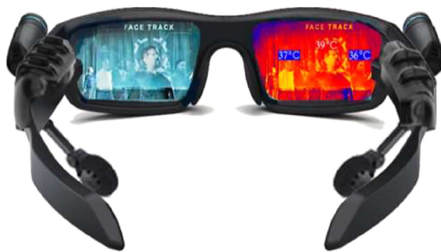
Figure 19: Smart glasses temperature capturing (Mohammed et al., 2020).
