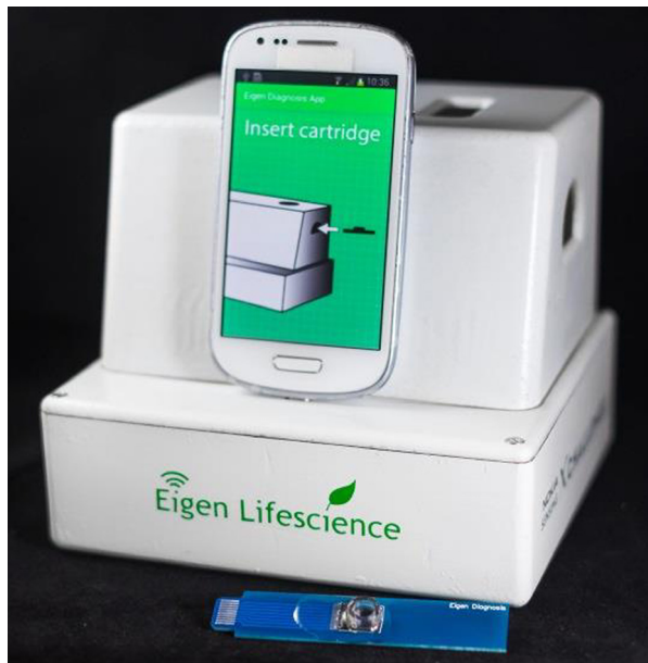
Figure 3: Picture of GMR-based portable device reported by the researchers from Stanford University (Choi et al., 2016).
