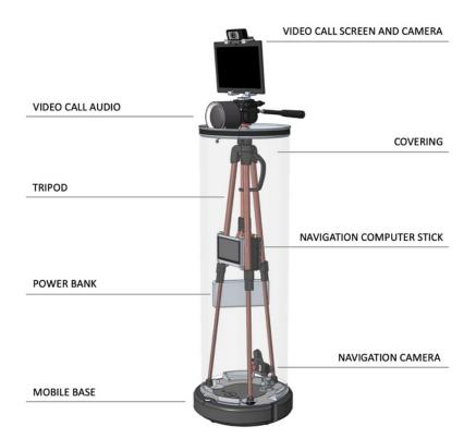
Figure 5. The LHF Connect teleoperated robot.
