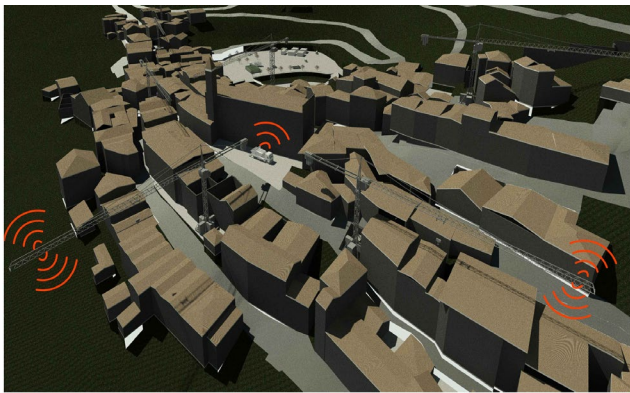
Figure 1. Rendered view. The figure represents the BIM model of Fossa with the preparations for the construction site (crane, common storage area, etc.)
