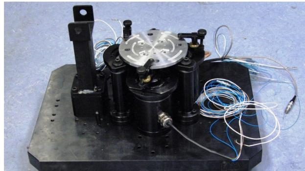
**Figure 1.** The proposed PKM fixturing system, (Maximum Volume as 6 dm<sup>3</sup>)
