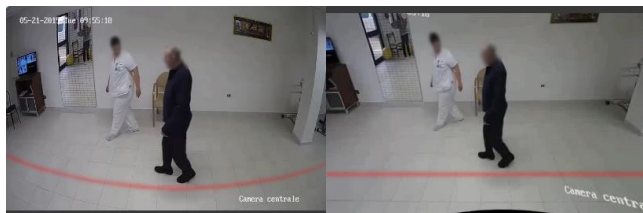
FIGURE 5. Before and after application of fish-eye removal algorithm
