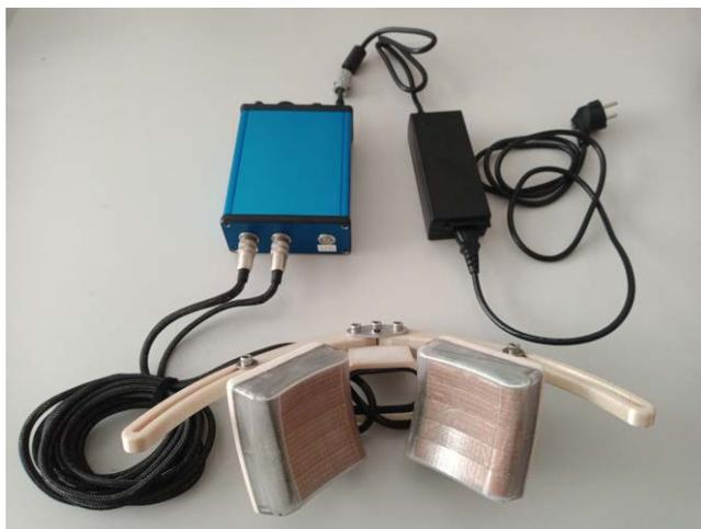
**FIGURE 1.** Transcutaneous Fetal Visual Stimulator. The device, FPGA-based and full-custom designed, comprises two displays that render complex visual patterns to fully cover the womb while enabling fetal measurements using an Ultrasound probe.
