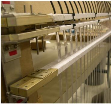
Fig. 11. A photograph of glued calorimeter optics including scintillating fiber ribbon, light mixer, and clear fiber bundle being cured in the assembly jig.
