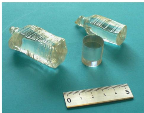
**Fig. 1.** Crystal boules #1 (left) and #2 (right) from which some improved samples studied in this work were obtained. The polished cylinder in the center, used to fabricate a scintillating bolometer described in Ref. [48], was obtained from a similar boule #3. The scale is in centimeters.
