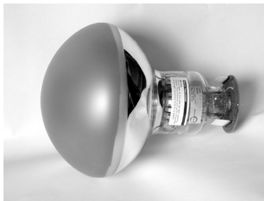
Fig. 1. 9357FLA Electron Tubes photomultiplier with blasted glass window.
