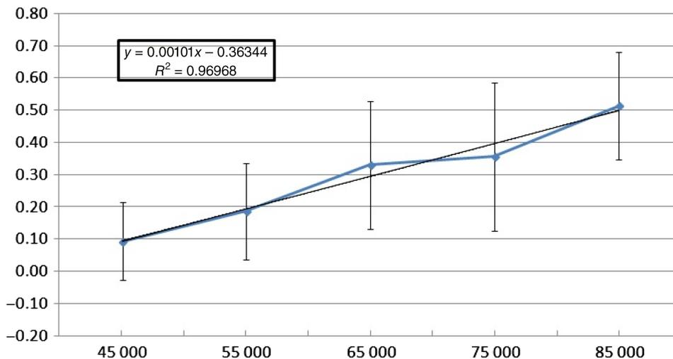
Figure 6. Pressure calibration points (*x*-axis) and differences between the readings of the sensor under calibration and the reference one (*y*-axis) with uncertainty bars and linear regression calculated as calibration curve.
