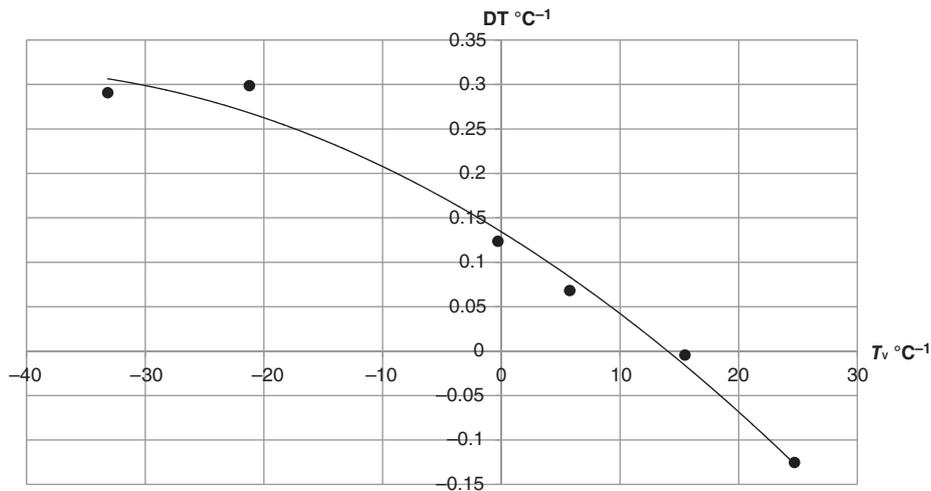
Figure 5. Calibration curve evaluated as correction function to be applied to the sensor readings as a function of the temperature.
