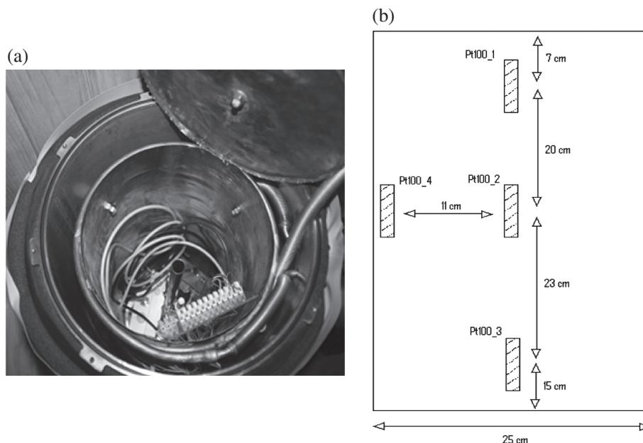
Figure 2. (a) Picture of the inner part of the chamber during the characterization procedure. (b) Scheme of the sensor positions inside the portable climatic chamber, during the characterization procedure.
