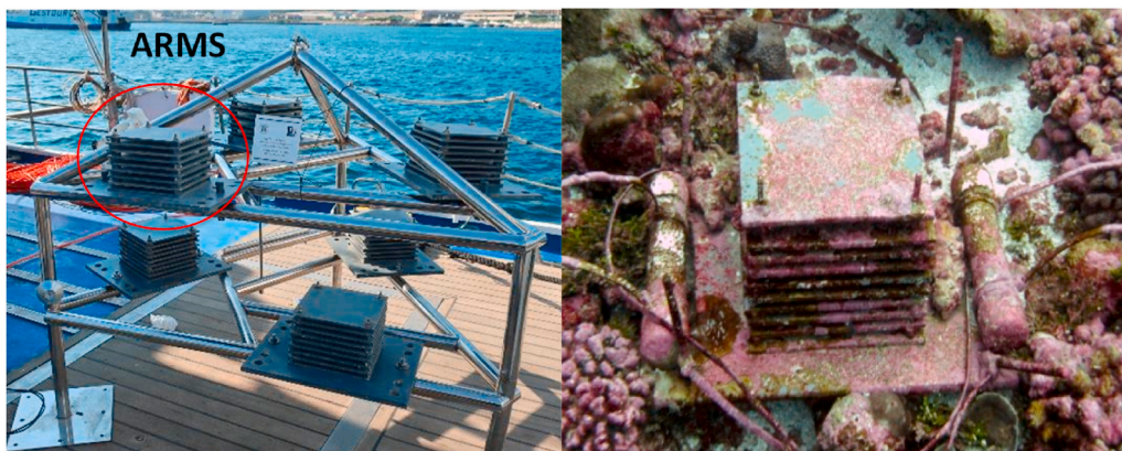
Fig. 2. The Autonomous Reef Monitoring Structure Unit (ARMS) before and 2 years after deployment. This is an example from the shallow water.
