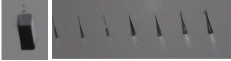
Figure 8. Rectangular and circular micro-holes developed in collaboration with TUM by means of a focused 17MeV proton beam. The pictures are taken under a tilted angle allowing to observe the internal conical surface profiles of the respective micro-structures.
