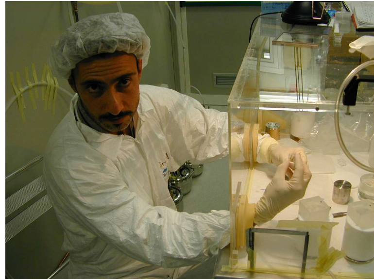
thermistor & heater gluing
