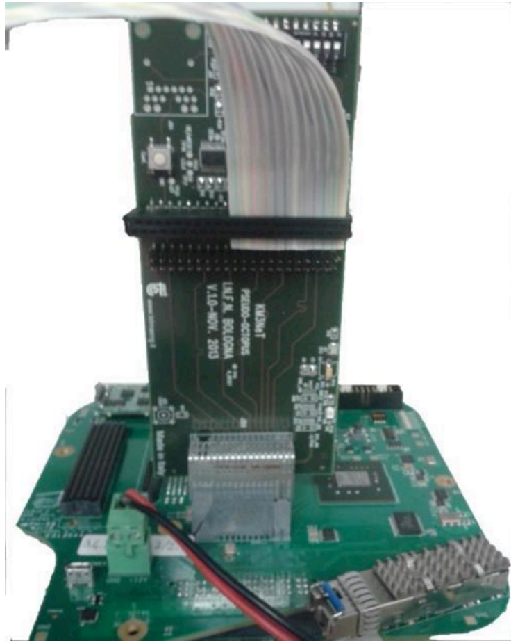
FIG. 7: Pseudo Octopus board plugged on a CLB
