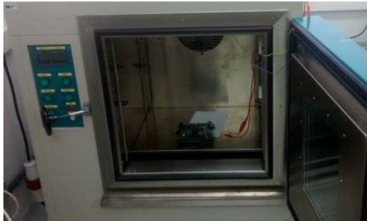
FIG. 13: CLBv2.2 inside the climatic chamber for the HALT test.
