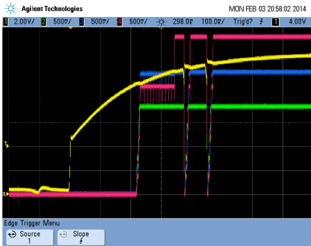
FIG. 14: Start up measurements on 1.8V (green), 2.5V (blue), 3.3V (red) and 12V (yellow), by using the "slow" power generator; several restarts were caused, which lead to the FPGA breaking.
