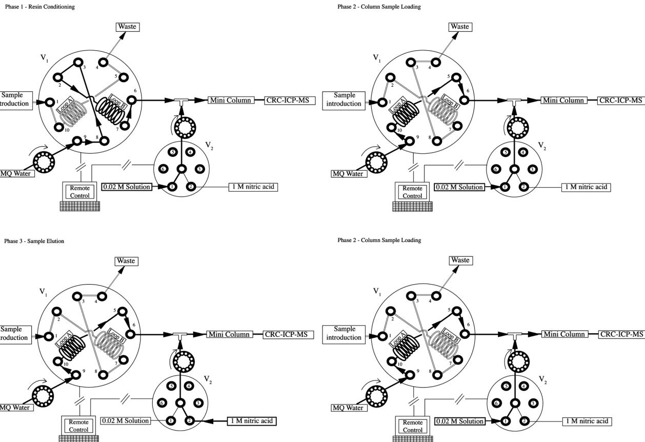
**Fig. 1** Schematic view of the flow injection manifold system for sample introduction to the CRC-ICP-MS. Solid lines indicate the path of fluid transport through the system ( $0.8 \text{ mL min}^{-1}$ ) while the hollow lines show the sample loading channel.
