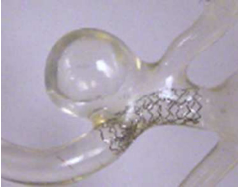
Fig. 1. An in vitro model of a cerebral aneurysm with a stent.
