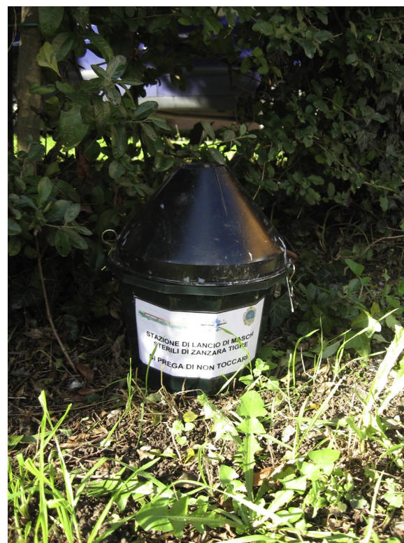
Fig. 2. Male pupae release station adapted with an inverted funnel on the top.
