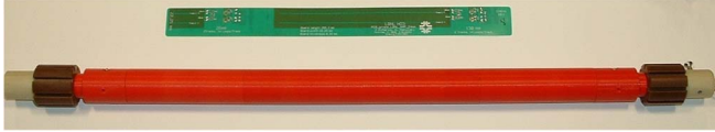
Fig. 2. PCB with both 26 and 130 mm long, 26 mm in diameter probes (top) and PSB probe holder (bottom). Typical probe rotational speed is 1 Hz.
