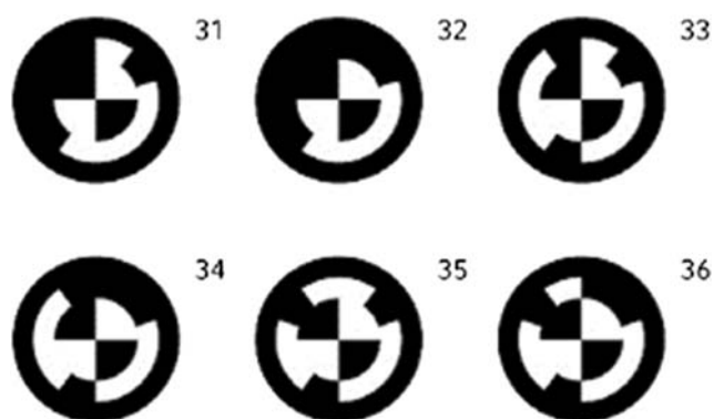
Fig. 8 Examples of artificial coded GCPs (Daftrey et al. 2015)
