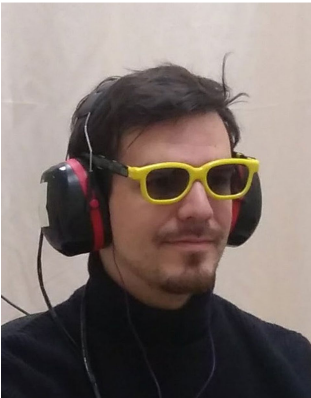
Fig. 5 A participant listening through the microphone arrays embedded in the Glassense device with noise isolating headphones, to avoid external sounds leakage
