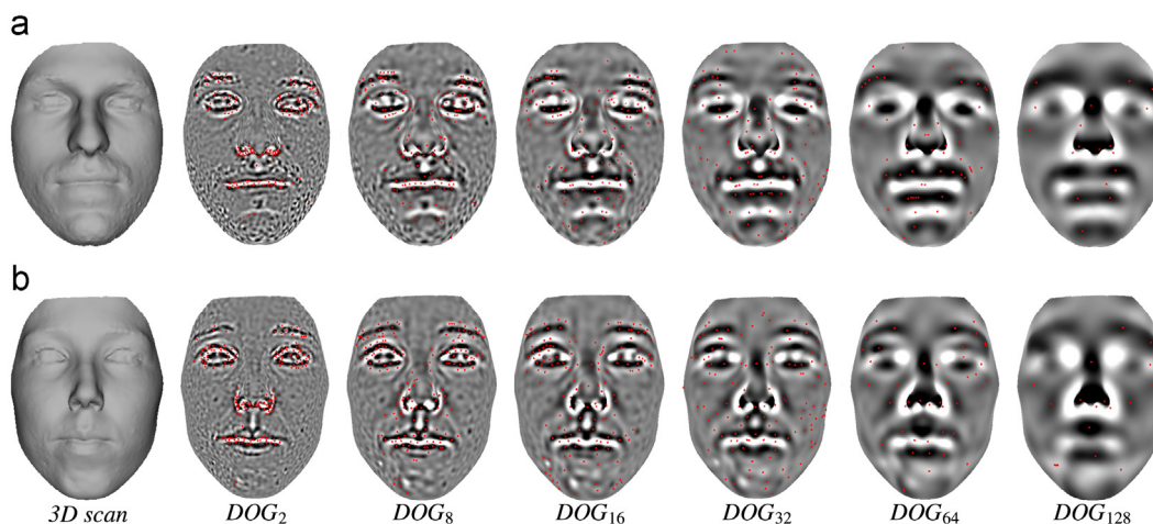
Fig. 2. DOG_k values at different scales and the 3D keypoints detected at that scale for a male subject in (a) and a female subject in (b). (a) subject002 and (b) subject003.
