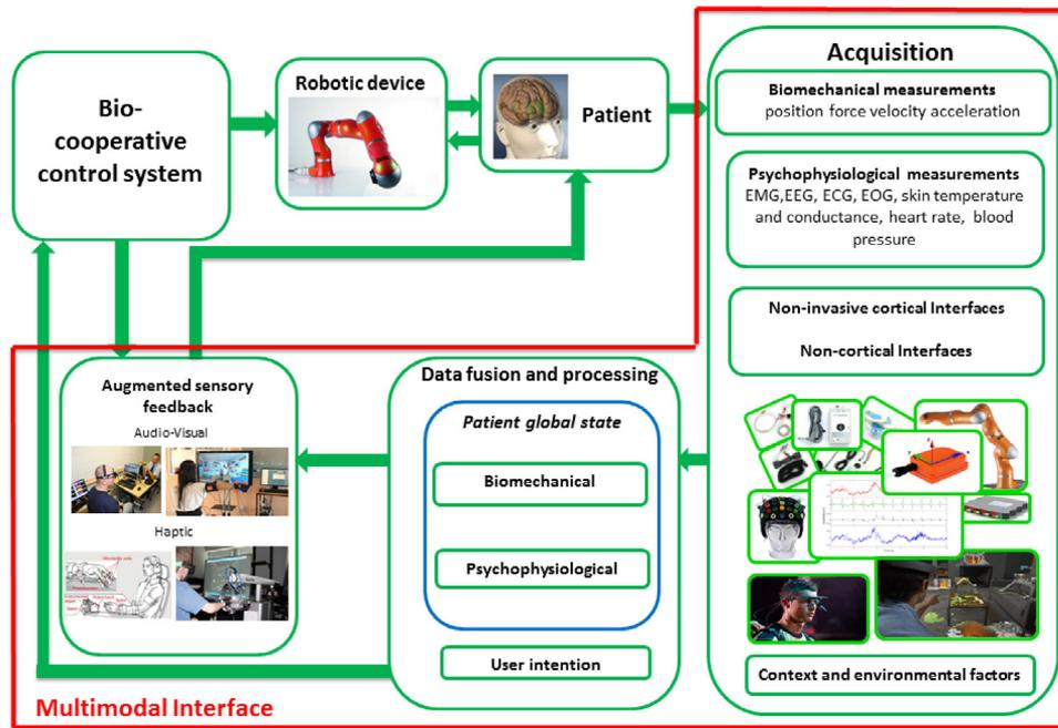
Fig. 1. Computational schema of the proposed bio-cooperative system for upper limb robotic rehabilitation.
