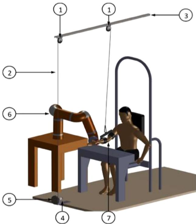
**Fig. 3.** Mechatronic module for arm weight support: (1) pulleys; (2) steel wire; (3) steel bar; (4) actuation system; (5) aluminum drum; (6) 7-DoF Kuka LWR; (7) forearm-belt support.
