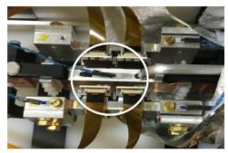
**Figure 2.** SDD detector (left) consisting of an array of 2x4 SDDs and the arrangement in the vacuum box of VIP2 (right). The white circle indicates the position of the X-ray detectors positioned on both sides of the water-cooled copper target conducting a current of about 100A.
