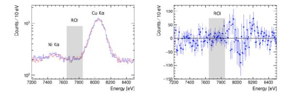
**Figure 3.** The X-ray spectrum measured with current and without current in VIP2 (left). The region-of interest (ROI) is shaded. After subtraction of the background events the residual X-ray spectrum is shown in the right panel.
