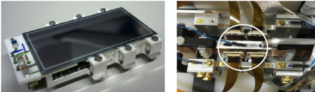
**Figure 2.** SDD detector (left) consisting of an array of 2x4 SDDs and the arrangement in the vacuum box of VIP2 (right). The white circle indicates the position of the X-ray detectors positioned on both sides of the water-cooled copper target conducting a current of about 100A.
