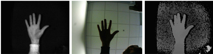
Fig. 2. Sample infrared, RGB, and depth images from the Briareo dataset. Samples have been acquired with a standard RGB camera and the Pico Flexx device.
