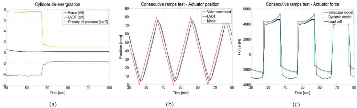
Fig. 2. Results of the tests on the legacy system.(a) cylinder de-energization procedure, (b) actuator position; (c) force matching during consecutive ramps test
