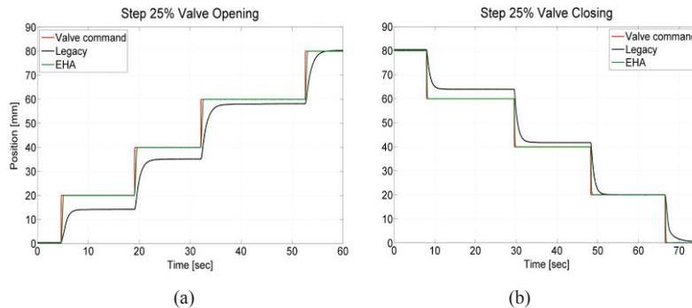
Fig. 3. Comparison of the accuracy of the Legacy and EHA systems on valve opening (a) and closing (b)
