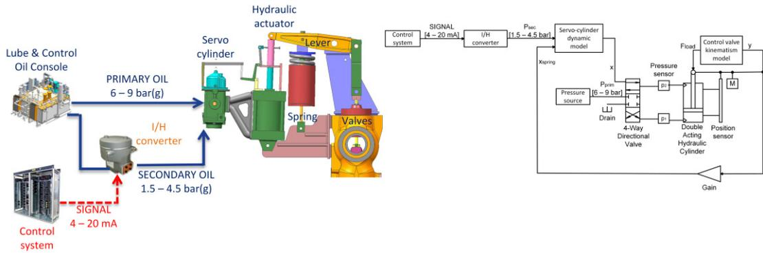
Fig. 1. (a) Legacy actuation system with control valve assembly; (b) Simulation model layout
