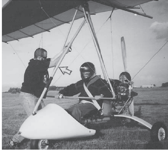
Fig. 6. Damped glider tube of Ołędzki et al. [11] (see arrow). Reprinted with permission from Elsevier.
