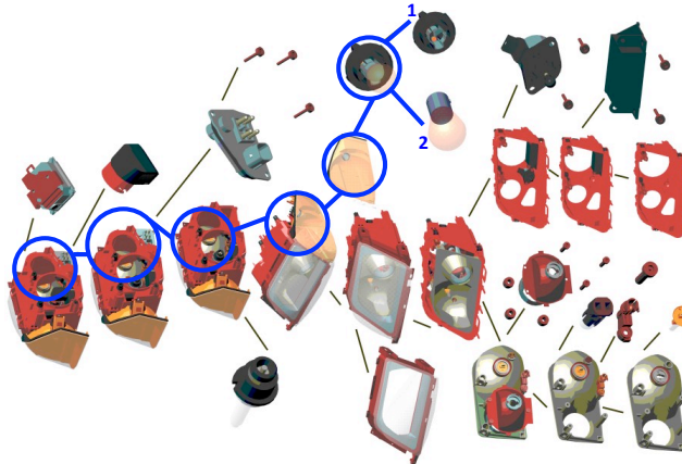
Figure 1: Precedence graph in dismantling operations: jobs 1 and 2 share the operations on the encircled parts.
