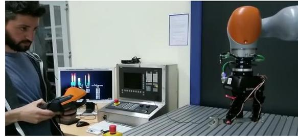
Fig. 9. KUKA LBR iiwa 7 R800 robot grasping a wrench. The pressure values at the fingertip are visualized on the monitor.
