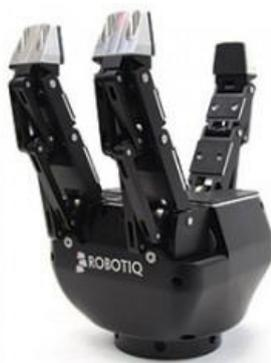
Fig. 1. 3-Finger Adaptive Robotiq® gripper [18].
