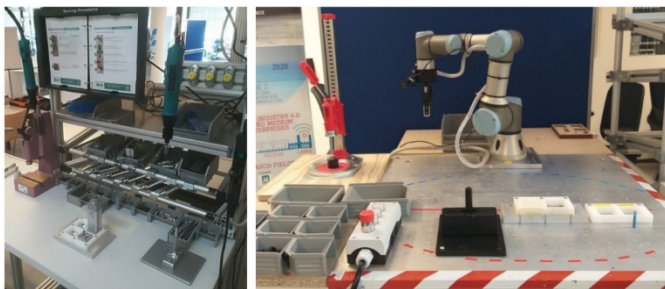
Fig. 1. Left: original manual assembly station of our case study. Right: toward a fully collaborative station based on the UR3 robot.
