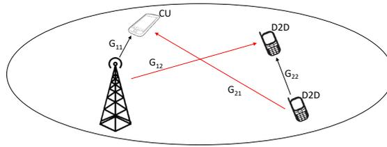
Fig. 1. Interference relations in the downlink. The cellular terminal (CU) suffers from interference produced by a D2D pair and viceversa.
