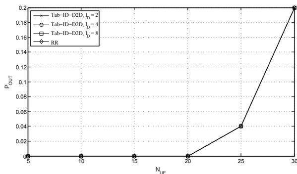
Fig. 4. Outage probability in presence of D2D NB-IoT pairs.
