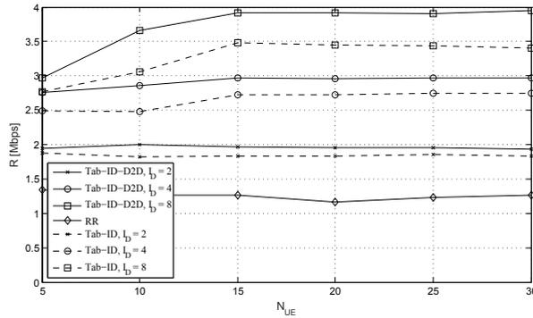
Fig. 2. Rate per cell as a function of the number of terminals in presence of 2 D2D NB-IoT pairs with the allocation strategies.
