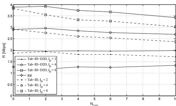
Fig. 5. Rate per cell as a function of the D2D NB-IoT number of pairs with the allocation strategies and  $N_{CU} = 20$ .
