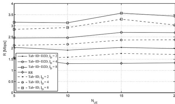
Fig. 3. Rate per cell as a function of the number of terminals in presence of 10 D2D NB-IoT pairs with the allocation strategies.
