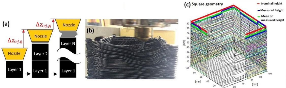
Fig. 3. Robot height **above** the optimal range: (a) Scheme of the effect caused by a too high commanded robot height; (b) Deposition defects in a real experiment using square geometry; (c) Deposition defect measured with laser sensor as error between nominal and measured layer height.
