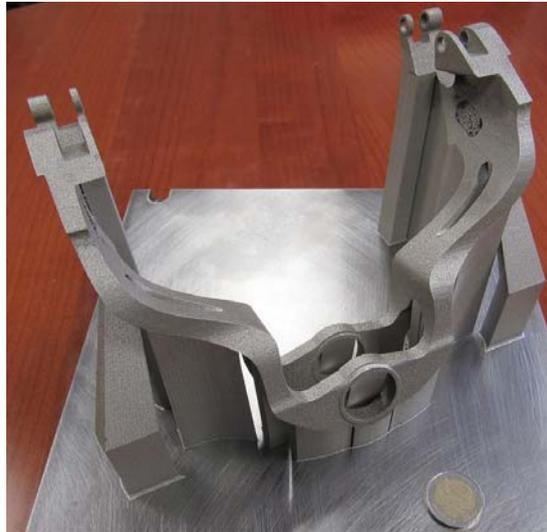
Fig. 10. The part, as manufactured, with anchor supporting on the building plate.
