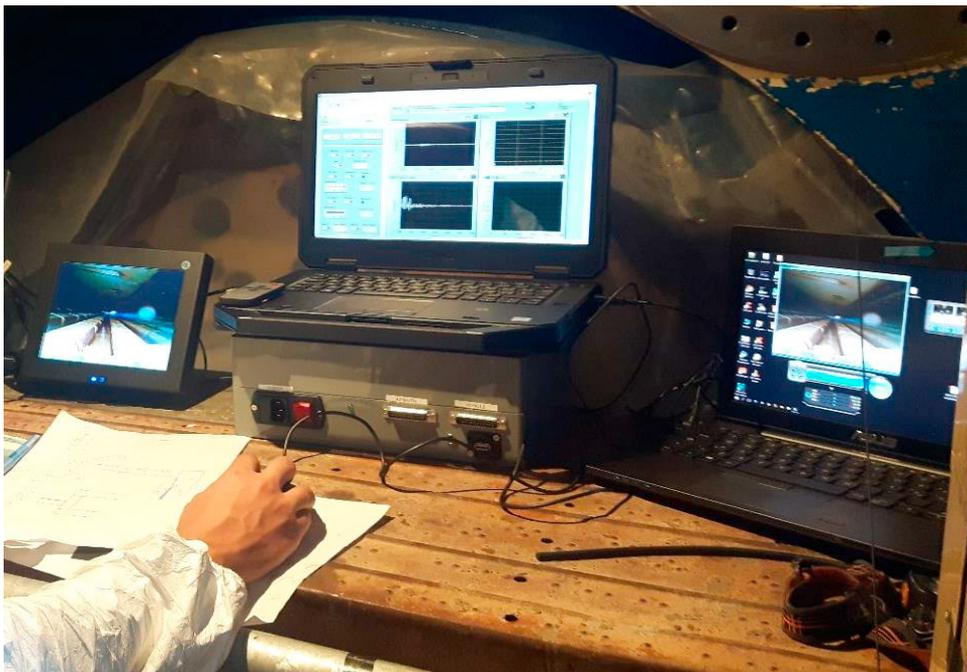
Fig. 5. Visual inspection testing with the crawler vehicle on a specific generator.
