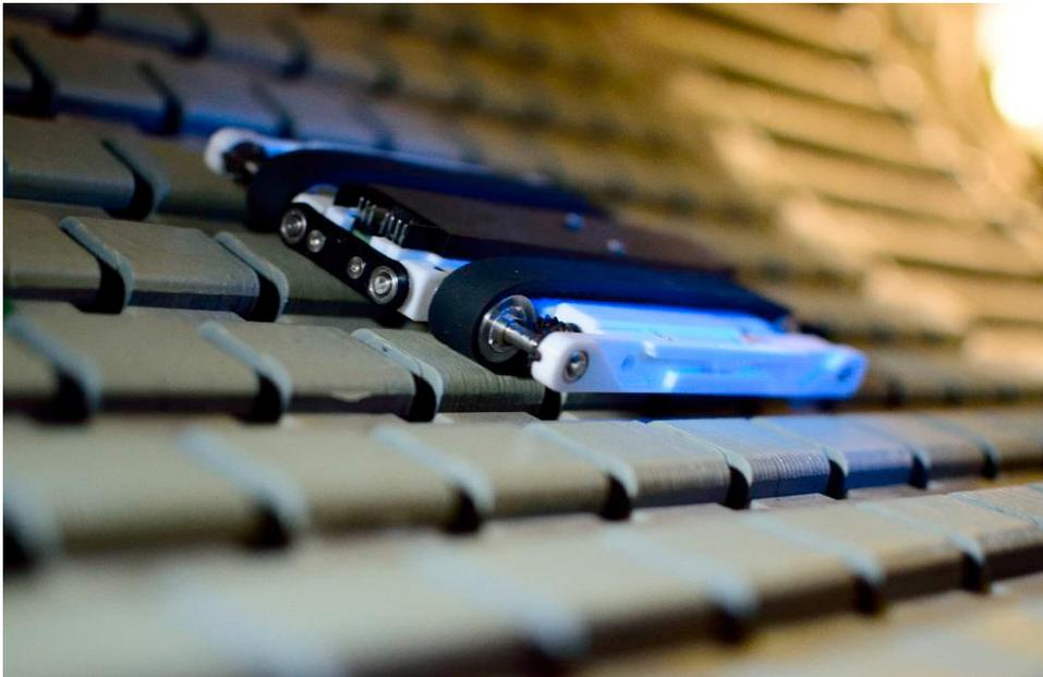
Fig. 4. The robot prototype crawling on the stator of an actual generator with the rotor removed.
