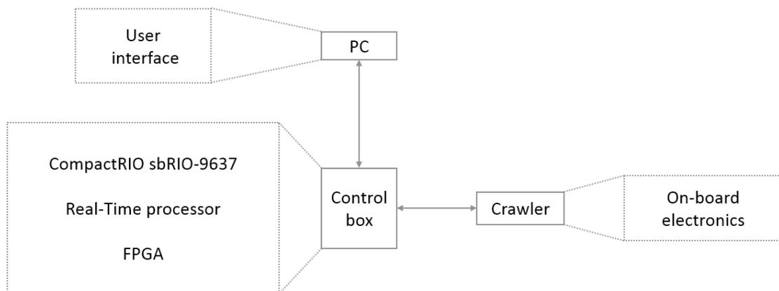
Fig. 2. Overview of the architecture of the inspection system.
