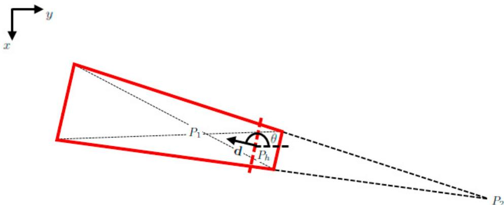
Fig. 3. Schematization of the pose estimation problem. On the Spanish fan (in red) are shown the main variables involved in the problem and the camera frame (in black).
