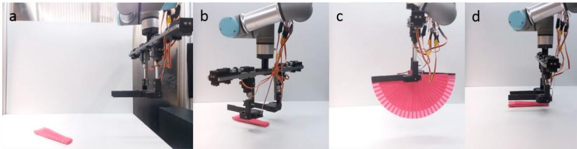
Fig. 4. Sequences of Spanish fan handling. (a) The Spanish fan is within the workspace in random pose. (b) The algorithm estimates the object pose and sends it to the UR3 arm, which moves toward those coordinates. (c) The gripper grasps the Spanish fan and handles it applying the velocities calculated in eq. 9. (d) The gripper releases the Spanish fan on the table before being moved to the starting position again.
