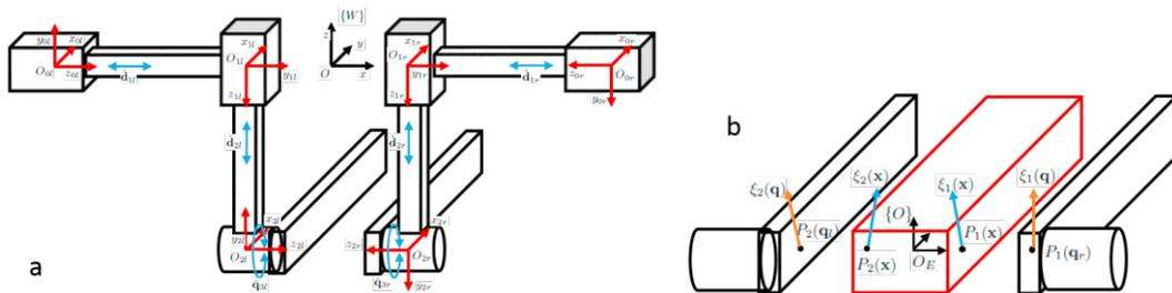
Fig. 2. (a) Gripper kinematic model: the world frame  $\{W\}$  (in black), the local frames  $\{O_i\}$  (in red), the joint velocities (in blue). (b) Dexterous manipulation problem: the twist  $\xi_i(x)$  of point  $P_i$  due to the twist  $\xi_E$  of the frame  $\{O_E\}$  (in blue), the twist  $\xi_i(q)$  of point  $P_i$  due to joint variables (in orange).
