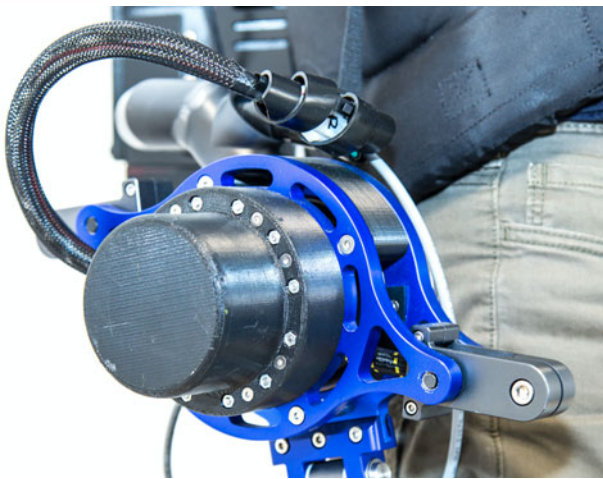
FIGURE 2 Picture of the parallel-elastic actuator on the Robo-Mate active trunk, described by Toxiri, Calanca et al., (2018). The spring is implemented with a bungee cord and acts in parallel to a gear motor, hidden by the black cover in this picture.
