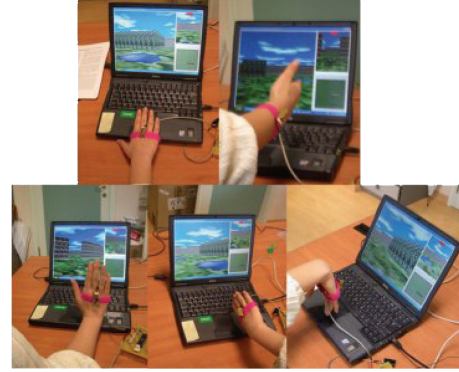
FIGURE 7: A set of screen captures of the virtual world, as seen from an LCD while a user is interfacing with it through MOCA.
