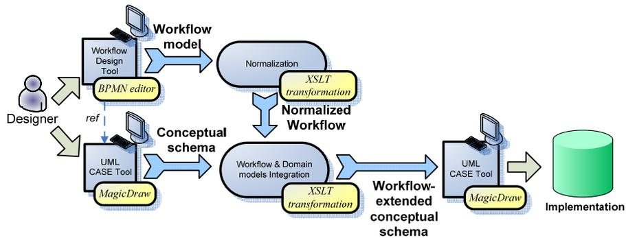
Fig. 12. Tools used for the MDD generation of Workflow-extended conceptual schemas.
