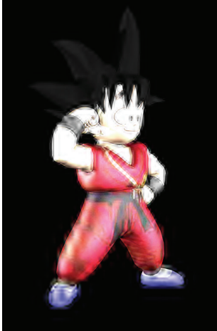
FIGURE 12: View of the Goku model corrupted by a loss in the first part of the texture codestream.
