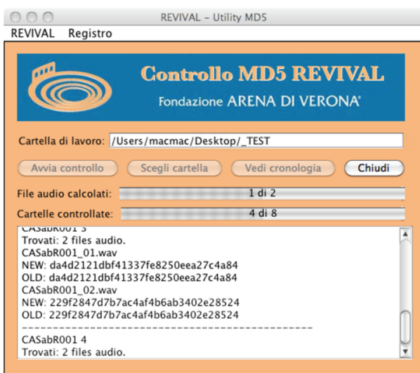
FIGURE 8: One of the software tools developed for the Fondazione Arena di Verona. This utility performs a consistency control on the checksums of the stored preservation copies and should be run periodically. The utility processes the entire archive of preservation copies and outputs a log in real-time, informing the operator about the remaining time by means of two progress bars (one for the number of preservation copies and one for the single audio files). The output on the screen reports the files that are being processed at the moment: in case of a mismatch between the checksums, an alert message is notified to the operator.
