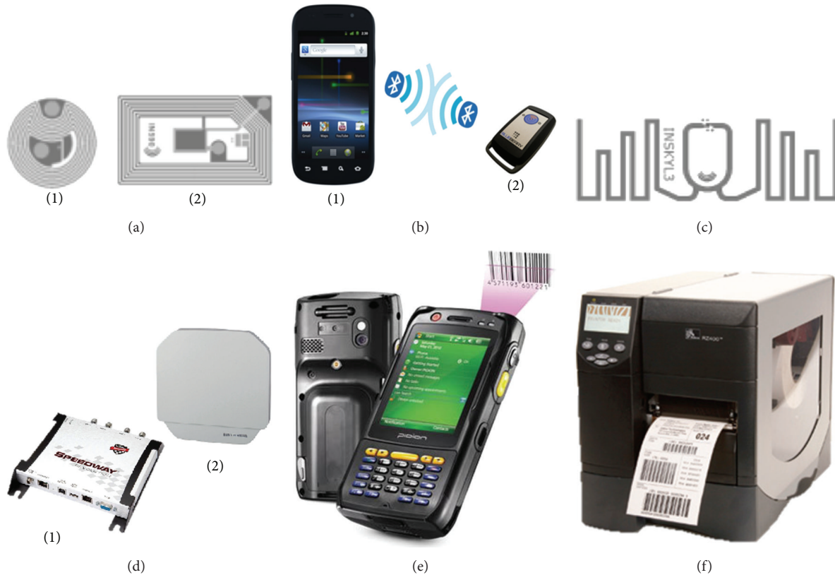
FIGURE 4: Main devices used in the pilot Project: (a) NFC tags: (1) Mifare Ultralight and (2) Mifare Classic; (b) portable NFC/RFID scanner composed of a (1) Samsung i9023 Nexus S and a (2) BlueBerry reader; (c) INSKYL3 passive UHF RFID tag; (d) RFID UHF gate composed of (1) Impinj Speedway Revolution R420 reader and (2) Wide Range UHF Kathrein antenna; (e) BIP-6000 of Meteor scanner; (f) Zebra RZ400 printer.
