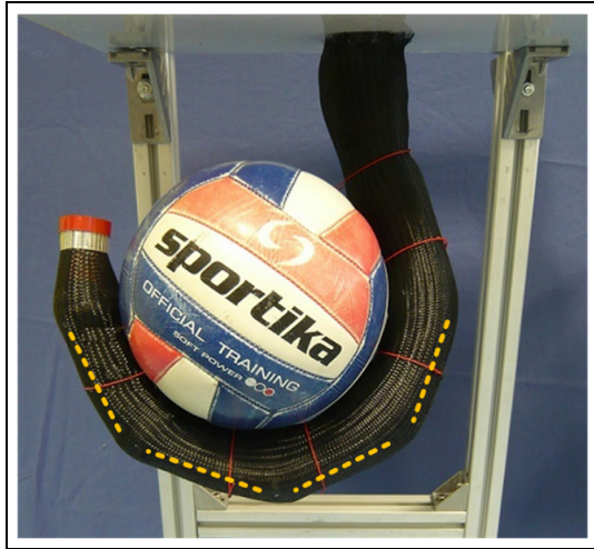
Figure 9. The arm prototype is grasping a ball. The activated PMAs are indicated with the dashed yellow lines.
