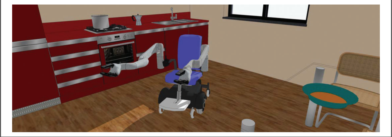
Figure 2. Concept of the wheelchair with two manipulators within an AAL scenario.
