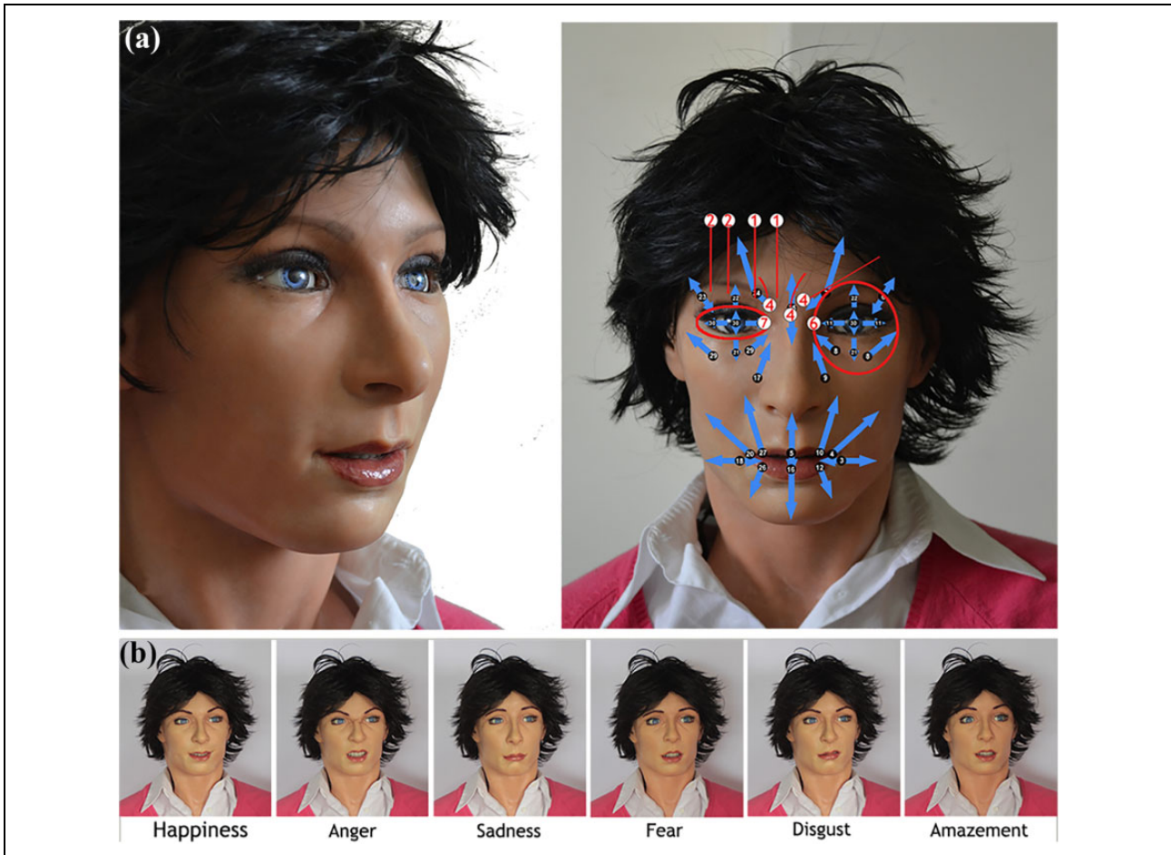
Figure 1. (a) The robot FACE (left), the major facial muscles taken into consideration (middle), and the servomotors positions inside the skull with an example of mapping between servomotor positions and action units of FACS (right); and (b) basic facial expressions performed by FACE. FACE: Facial Automaton for Conveying Emotions; FACS: Facial Action Coding System.
