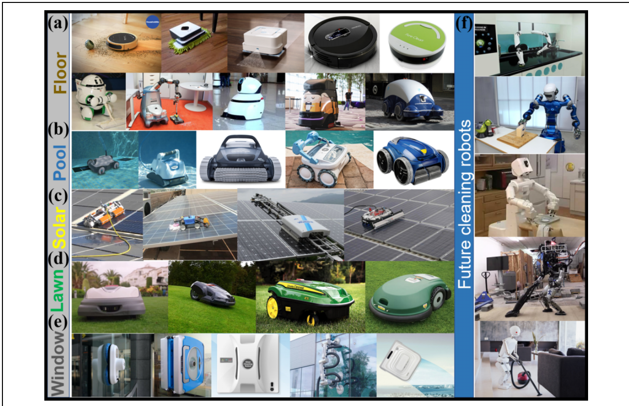
Figure 1. Commercial cleaning robots: (a) floor cleaning robots, 2–13 (b) pool cleaning robots, 14–17 (c) solar panel cleaning robots, 18–21 (d) lawn cleaning robots, 22–25 (e) window cleaning robots, 26–29 and (f) future multipurpose cleaning robots. 30–34
