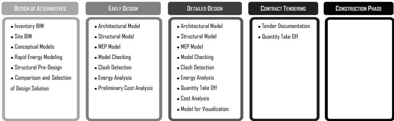
Figure 1. BIM design phases according to "Common BIM Requirement".
